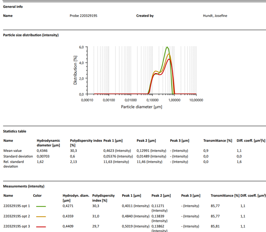
Figure 5: Dynamic Light Scattering for hydroxylated fullerenes.
