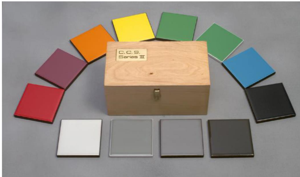
Figure 8-4: The Set of Twelve Calibrated Reflecting Ceramic Tiles, Produced by Lucideon Limited
